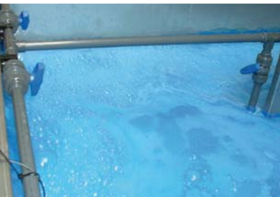
Long slow-down and flotation zone for optimal flotation of coagulated paint residue and clear water.
