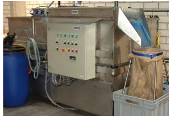
PolyFloat 3000 with removal of paint sludge in a jute bag.
