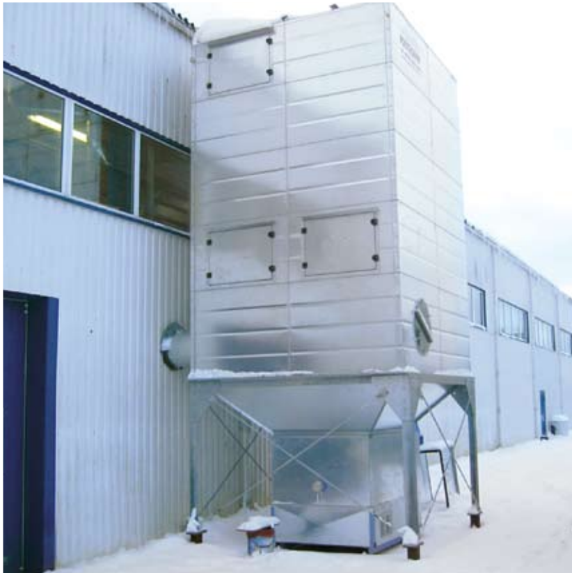
BrikStar C with protective housing, installed under a Höcker Polytechnik filter installation.
